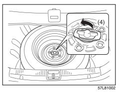
To remove the spare tire, remove the luggage under-box (2) and turn the bolt (4) counterclockwise.
